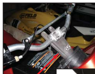
Aftermarket Bars Installed - OEM Protective Cover No Longer Fits
